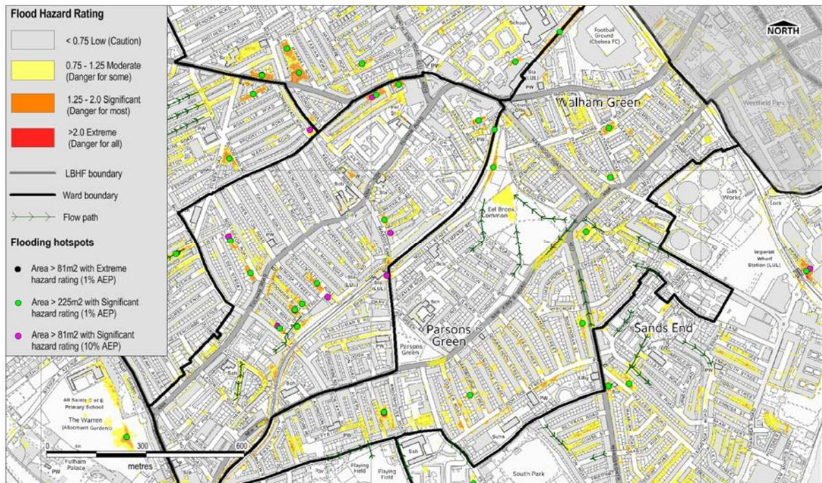
Figure 3.8-30 Parsons Green and Walham 1% AEP maximum modelled flood hazard
