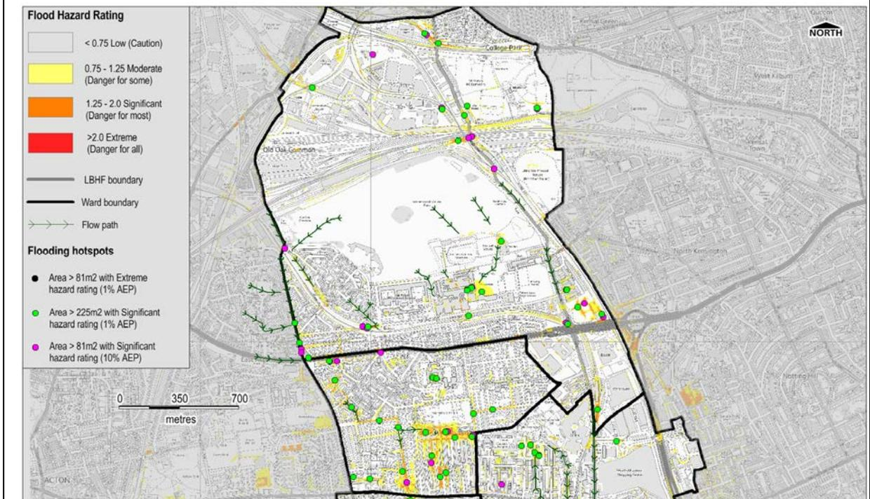
Figure 3.8-2 College Park and Old Oak 1% AEP maximum modelled flood hazard
