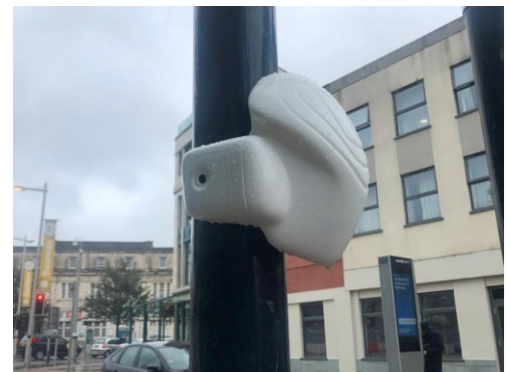
Vortex Air Sensor attached to a lamppost in Hammersmith & Fulham
