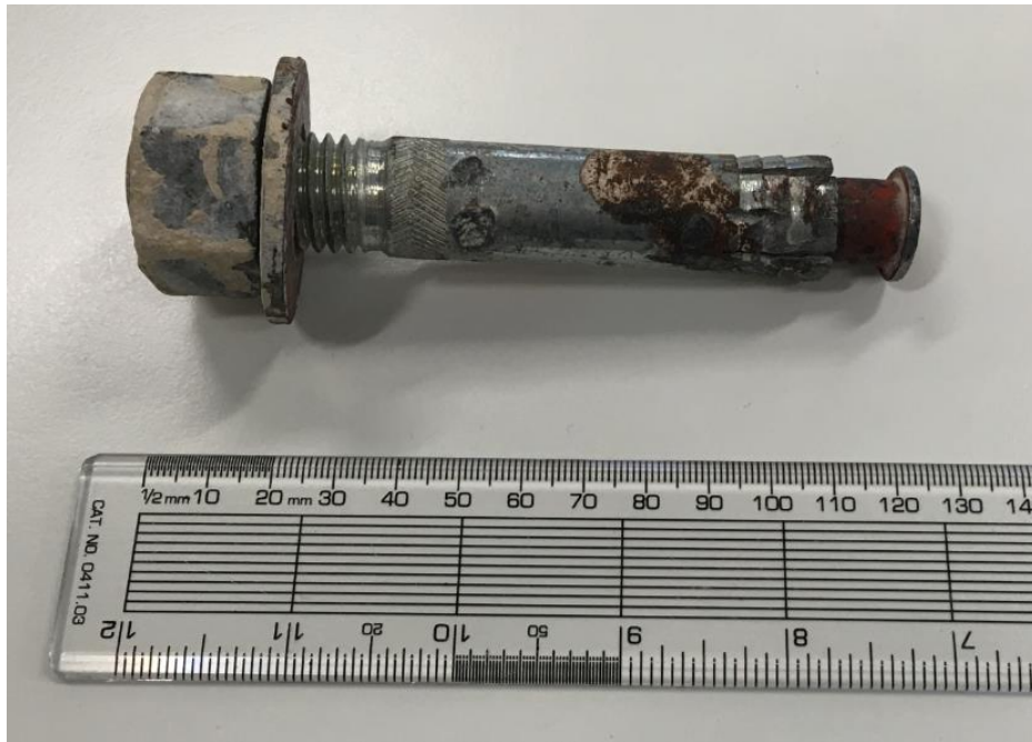
Figure 5 – One of the post-fixed anchors (assembled).
