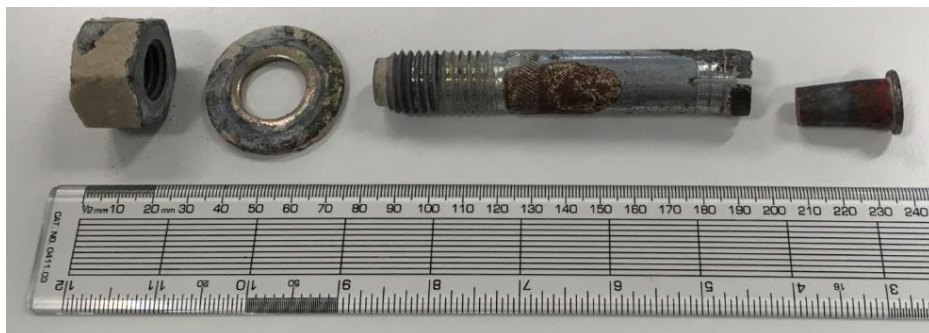
Figure 6 – One of the post-fixed anchors (disassembled).
