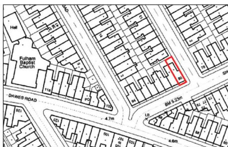
**Existing and proposed site plan:** This will show how the building or buildings are arranged on the site now and how they will be arranged if the proposals are approved or built. This is taken as an aerial perspective, looking down on the site.
