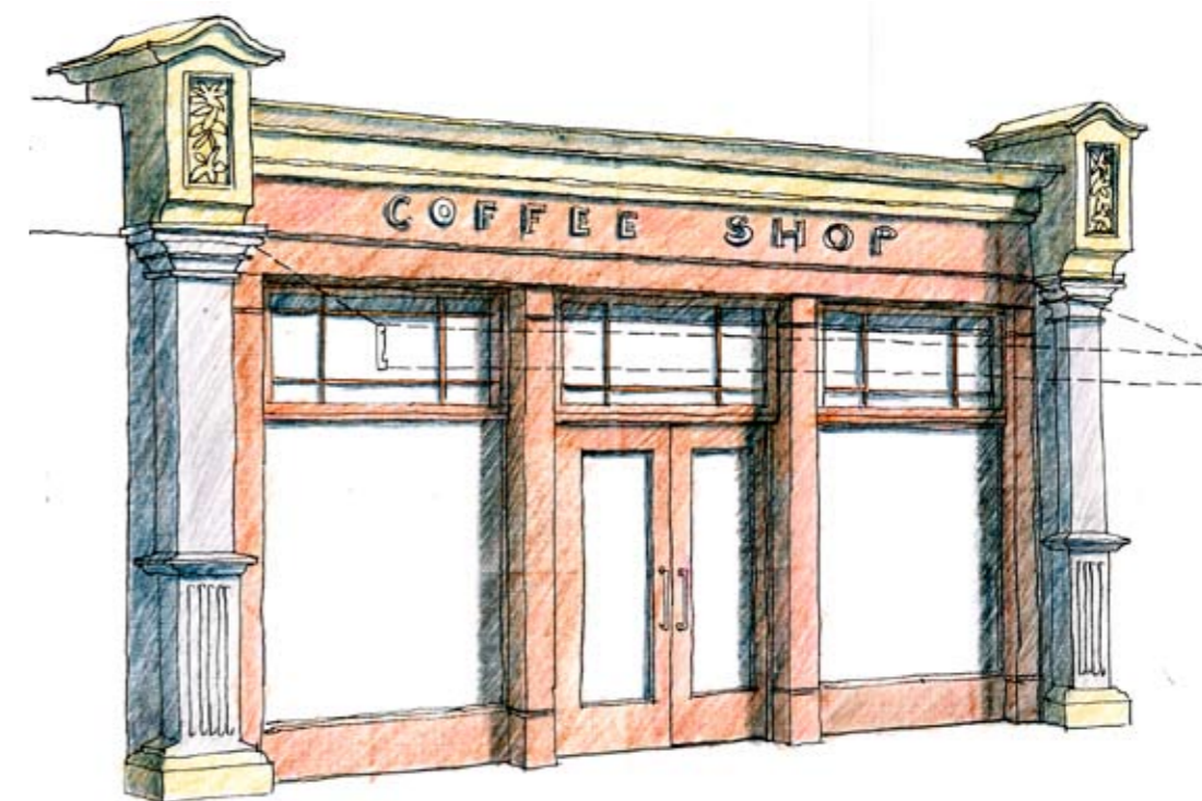
Appropriate example of a timber shopfront with centrally located doors within a restored shop surround
