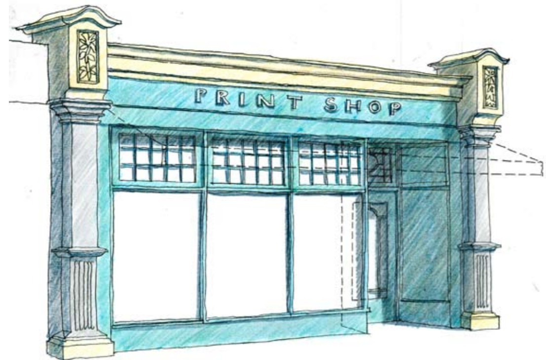
Appropriate example of a timber shopfront with recessed entrance door within a restored shop surround
