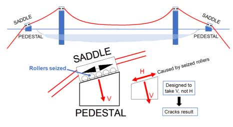
The suspension chains are subjected (red) to temperature changes which causes them to contract That and expand. is movement accommodated by rollers. Once the rollers seized, loads (H) were applied to the pedestals that they were not designed to take, and cracks in them resulted.
